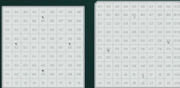
Example of a 81 vial (9x9 / left), and a 100 vial (10x10 / right) cryo box layout
