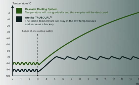
In the event of any failure with one of the cooling cycles, the other system will still maintain the temperature at a minimum of -70 °C. This means that your samples will not be affected by any challenges caused by an unexpected failure until service is provided.
