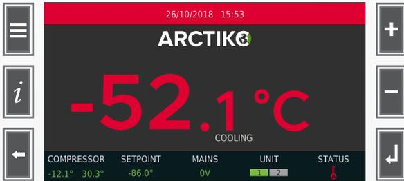
If the temperature in the unit rises above the “High temp” setpoint longer than the “Alarm delay” setting defines, the high-temperature alarm will be activated. If products with a temperature above the “High temp” setting are placed in the unit near the temperature probe, it may also trigger the high-temperature alarm.
