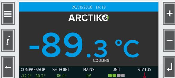
If the temperature in the unit falls below the “Low temp. alarm”-limit for a period longer than the “Alarm delay”, the low-temperature alarm is activated. In addition, if products with a lower temperature than the low-temperature alarm setting are placed against or close to the temperature probe inside the unit, it may also trigger the low-temperature alarm.
