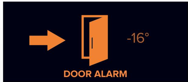
The unit is equipped with a door contact to register whether the door is open or closed. If the door is not closed correctly or held open for a period, the visual and audible “Door open alarm” will be activated. The alarm will stop when the door is closed correctly.
